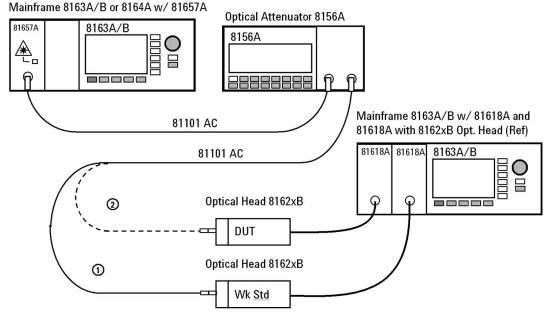
Figure 8 Accuracy Test Setup
