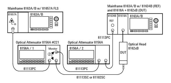
Figure 9 Measurement Setup for Power Linearity
