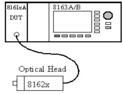
Figure 7 Functional Test Setup
