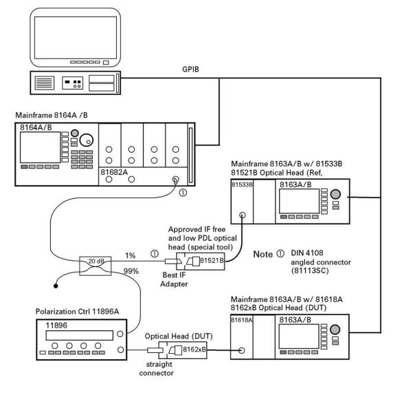
Figure 13 Measurement Setup for PDL Test
