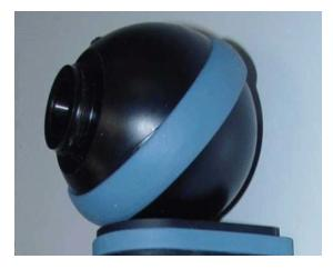
Figure 4 Attaching the Rubber Ring
