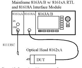
Figure 12 Return Loss Measurement Setup
